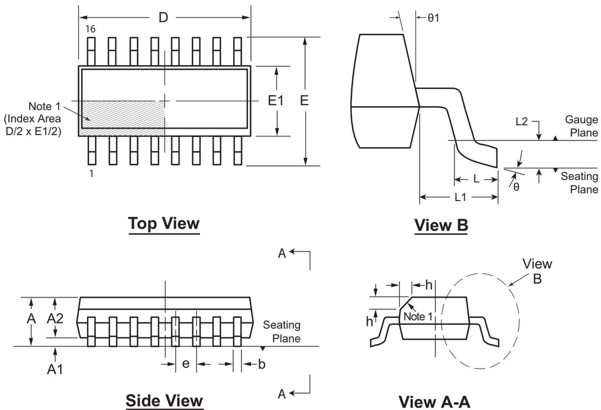
**Note 1:** This chamfer feature is optional. If it is not present, then a Pin 1 identifier must be located in the index area indicated. The Pin 1 identifier may be either a mold, or an embedded metal or marked feature.
